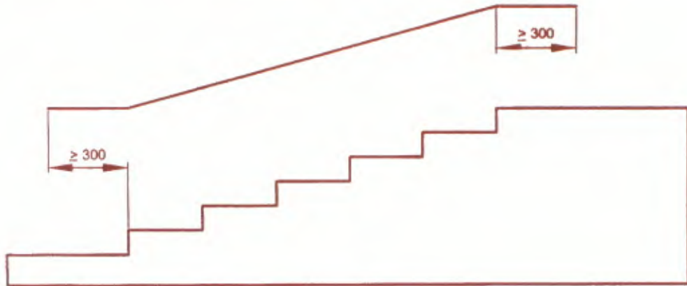
FIG. 16 EXTENSION OF HANDRAIL IN STAIRS
