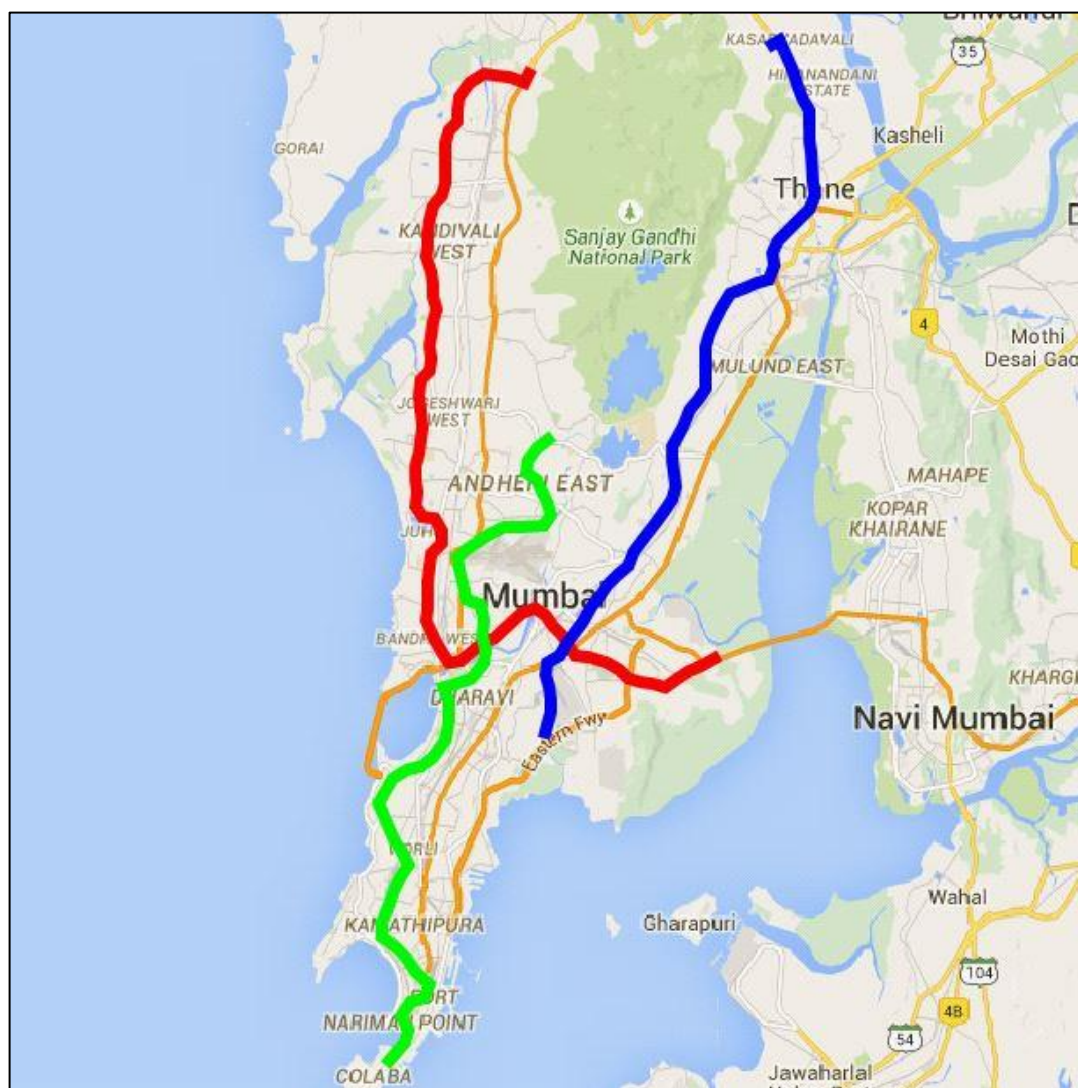
Figure 3.13: New alignments of Line “Dahisar-Charkop-Bandra-Mankhurd” (red line), Line “Colaba-Bandra-SEEPZ” (green line) and Line “Ghatkopar-Thane” (blue line)
